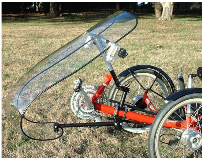
Greenspeed GTO with OnePoint mount and Forward Swing Feature.
